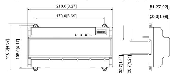
Figure 1-2 Dimensions (two-door two-way/four-door one-way) (mm [inch])
