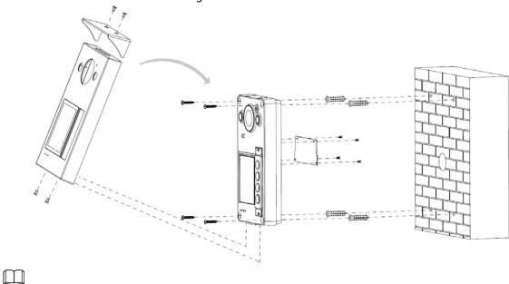
If you do not want to install the rain cover, you could use the sticker included in the package to cover the screw hole.
