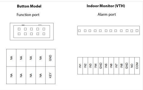
Connect the KEY port of the button model to any one of the alarm input ports of the indoor monitor (VTH) with a cable thread. After that, tap **Setting > Alarm > Wired Zone** on the VTH and set the **Type** of the alarm input port you chose to connect to the KEY port as **Doorbell.**
