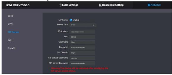
If other VTOs work as the SIP server, set Server Type as VTO, and then configure the parameters.
