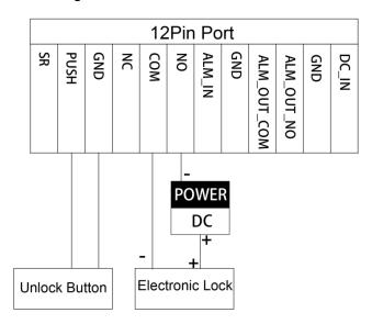
Figure 2-5 Magnetic lock connection
