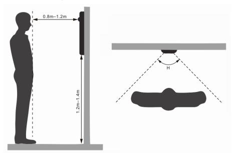
Figure 2-1 Installation position reference
