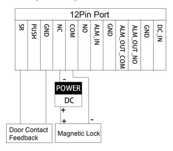
Figure 2-6 Electro-mechanical lock connection
