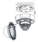
Figure 2-6 Secure the Camera
