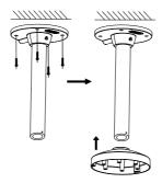
Figure 2-15 Install the Mount Bracket
