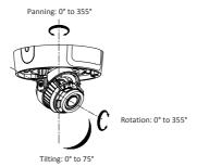
Figure 2-19 Adjust the Angle
