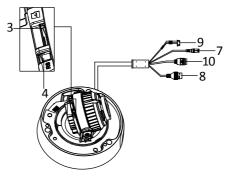
Figure 1-5 Cable Connection of Type IV Camera
