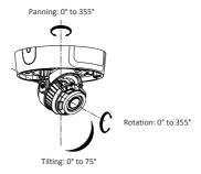
Figure 2-7 Adjust the Angle
