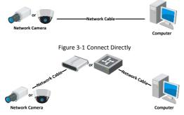
Figure 3-2 Connect via a Switch or a Router
