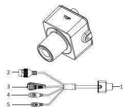
Figure 1-4 Overview of Type IV Mini Camera
