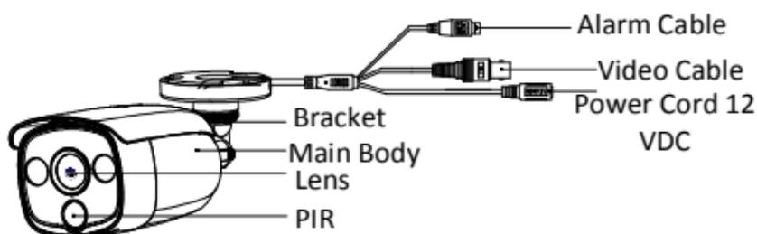
Figure 1-2 Overview of Type II Camera Installation
