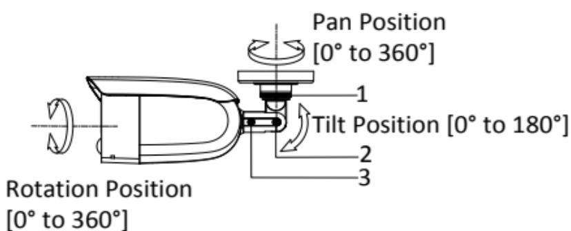
Figure 2-10 3-Axis Adjustment
