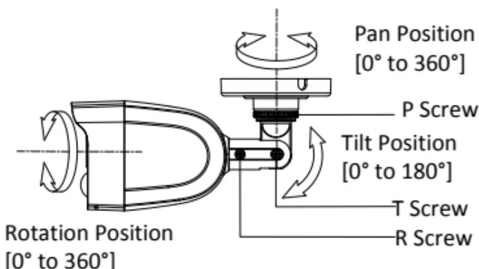
Figure 2-3 3-axis Adjustment
