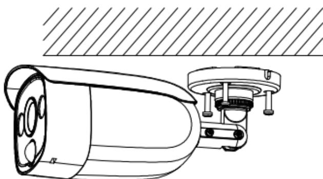
Figure 2-9 Install the Camera to the Ceiling
