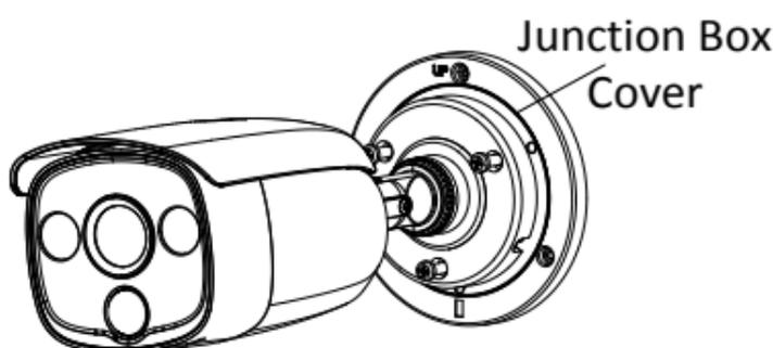
Figure 2-12 Install the camera on the Junction Box
