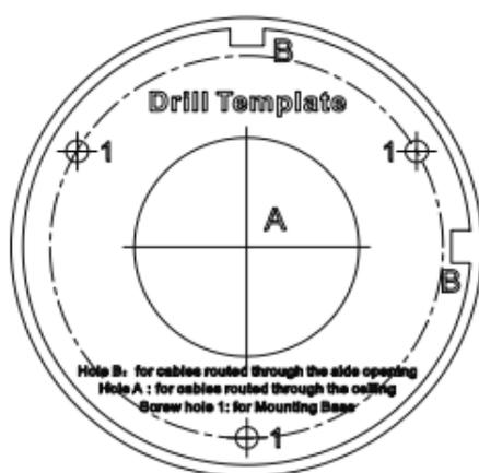
Figure 2-4 Drill Template of Junction Box
