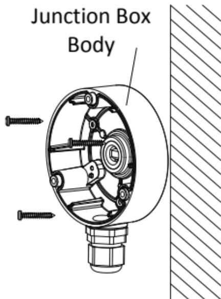
Figure 2-6 Secure the Junction Box to the Wall/Ceiling
