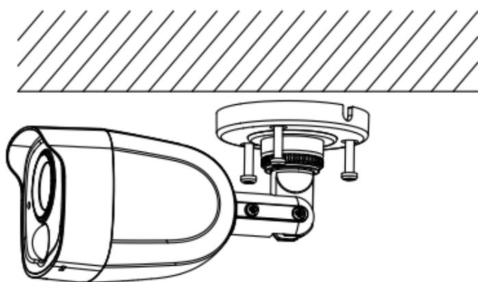
Figure 2-2 Fix the Camera to the Ceiling
