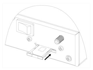
Figure 2-6 Install Card Slot
