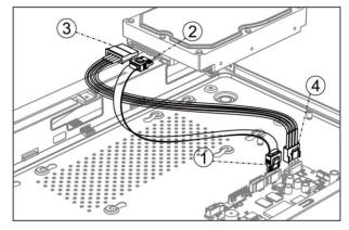
Figure 2-2 Connect Cables
