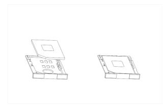
Figure 2-9 Install the SIM/UIM Card
