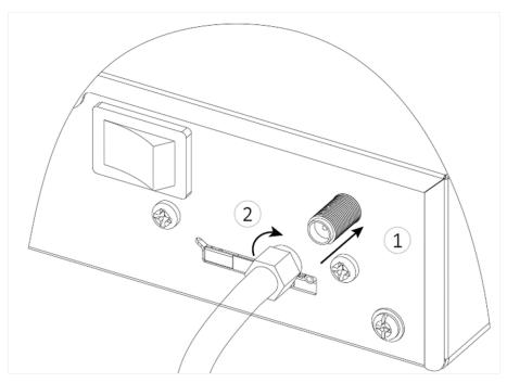
**Figure 2-11 Antenna Installation** 3. Put the antenna to a magnetic place with good signal. The antenna has magnet at the bottom.
