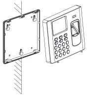
Figure 3-5 Install Front Cover
