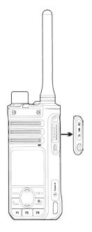
2. Insert the audio accessory plug into the accessory connector.
