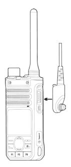
3. Tighten the screw on the audio accessory plug.
