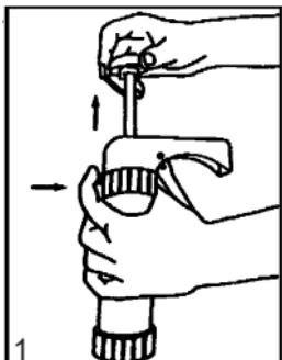
1 Press in metal locking device (near bottom of cylindrical part of cookie press) while pulling top knob.
