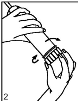
2 Unscrew bottom ring to insert dough into cylinder of cookie press
