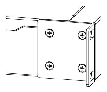
The device is designed to use indoors and it can be mounted in a rackmount enclosure using provided rack mounts, or it can be placed on the desktop. Please attach rubber pegs on the bottom of the router if the desired placement is on the flat surface or use a Phillips screwdriver to attach rackmount ears on both sides of the device if the designated use is for rackmount enclosure.
