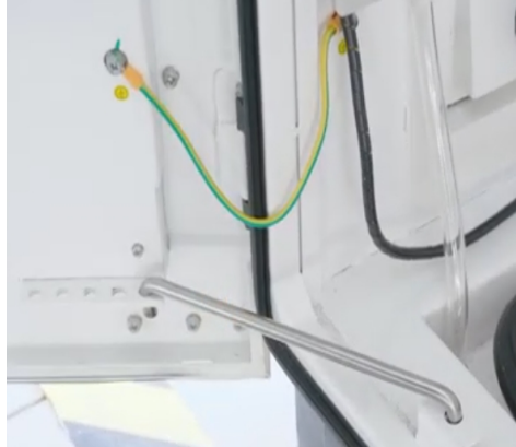
Figure 7- 10 Door stopper position
